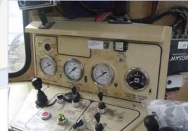
In cab filter element blockage display
