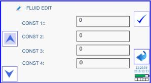
Save the setup through the tick button. Use the Return button to go back to the Test Point screen.
