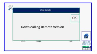
If the remote version is newer then the PCM500 will automatically upload the version to program memory.
