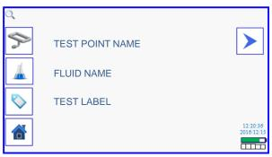
For example, if either the Test Point or Fluid buttons are pressed the screen will change to allow individual editing through buttons appearing to the right of the screen. Using the Test Label button will open the QWERTY keyboard.
