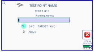
Important: The PCM can tolerate a 1°C per minute change in sample temperature during a measurement cycle. It is
