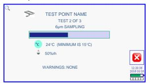
Should any test parameters be exceeded during a test a 'Warnings Present' label will be shown at the bottom of the screen. These will be recorded in the final result details screen.
